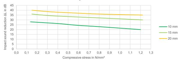
Due to the homogeneity of the material structure of matteco elastomeric bearings ELR 8, a relatively constant structure-borne sound insulation is achieved over a wide load range. This enables us to offer planners, architects, construction companies and building owners the greatest possible acoustic safety.
