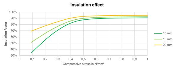
Shown is the insulating effect of ELR 8 at an excitation frequency of 100 Hz.
